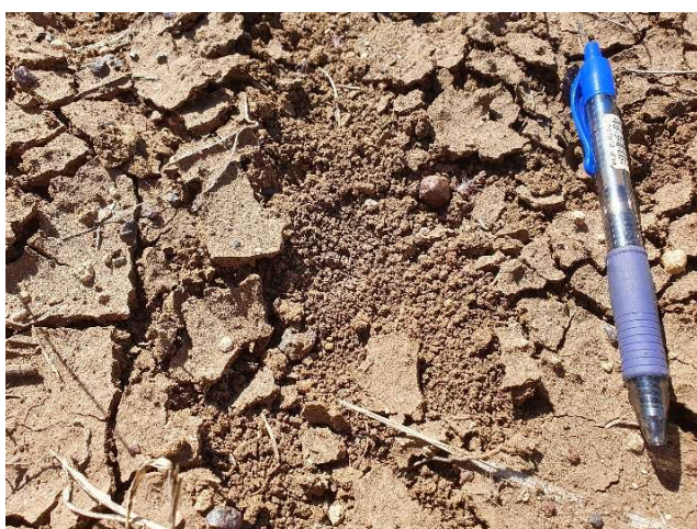
An easily disturbed surface crust on a clay soil. While this crust can be separated from the soil profile with ease, a layer of the underlying soil remains bound to the crust (AB)
