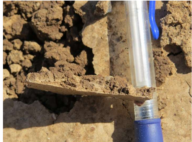
A thin surface crust on a cracking clay soil. The inability to separate the crust from the underlying soil is clearly visible (AB)
